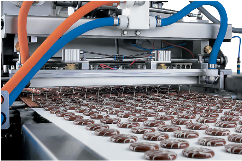
Figure 14.23 Picture of decorating machine. Source: Sollich. Reproduced with permission of Sollich Germany.
