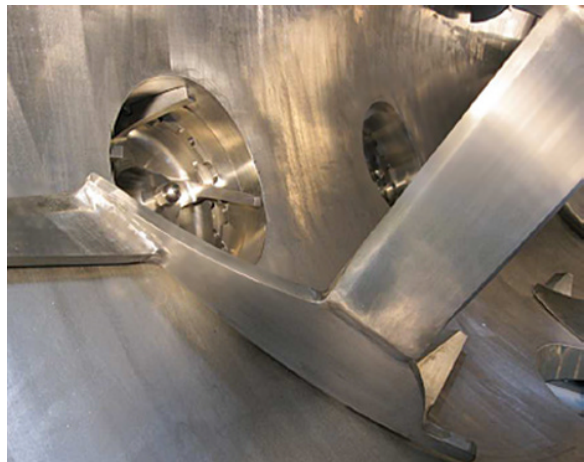
Figure 10.25 ECO 2 -Choc conche vessel with integrated grinding areas (Lipp Mischtechnik GmbH).
