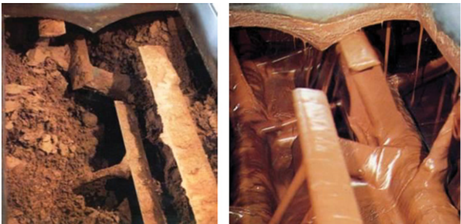
Figure 10.15 Conching paddles and mass consistency in dry and liquid phases inside HOMEGA conche. Source: Reproduced with permission of Carle and Montanari-OPM.
