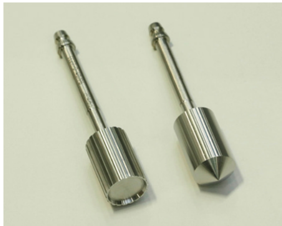
Figure 11.11 Bob types for concentric cylinder viscometers.
