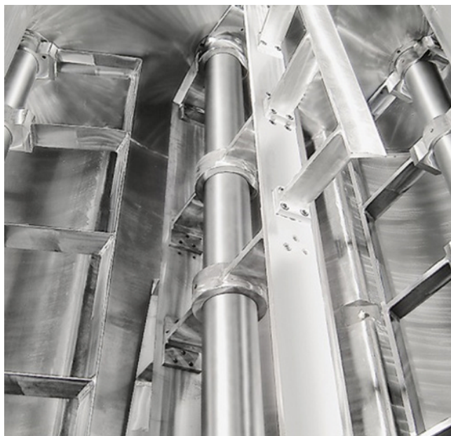
Figure 10.18 Conching paddles inside Frisse-DUEC conche. Source: Reproduced with permission of Bühler AG, Switzerland.
