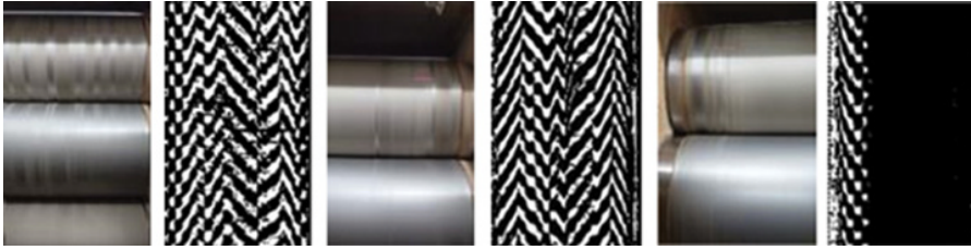
Figure 24.19 Different black-and-white patterns (whole roll length) for different incorrect control adjustments. Black is covered, white uncovered roll. Reproduced with permission of Bühler, Uzwil, Switzerland.
