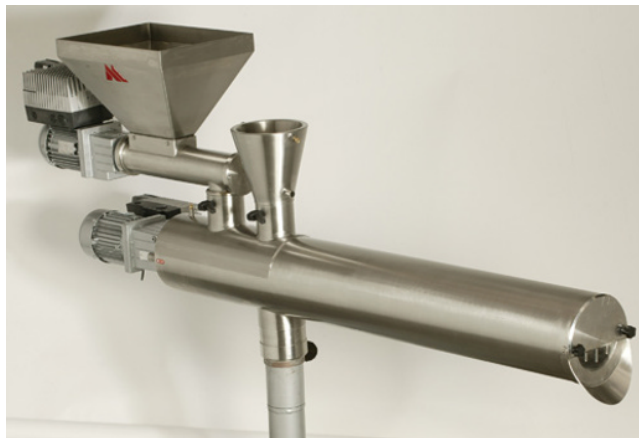
Figure 14.6 Screw mixer conveyor system. Source: Aasted. Reproduced with permission of Aasted Denmark.
