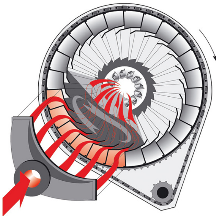
Figure 3.7 Schematic diagram of the heated gas flow within a JND Continuous Rotary Louvre Roaster. (JND Technologies Limited, Retford, UK).
