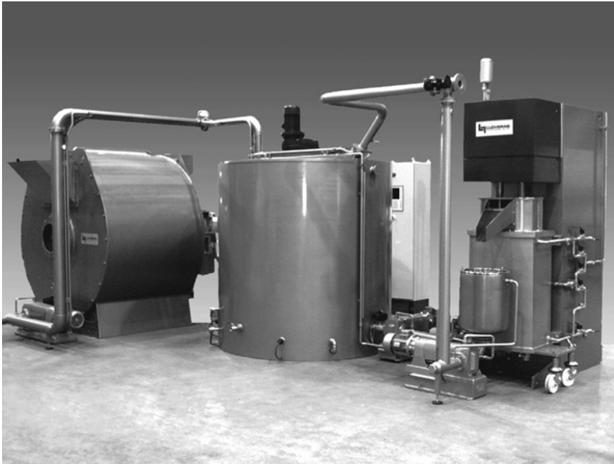
Figure 19.1 Lloveras Unicom system combining a refiner conche with a ball mill. Source: Aasted. Reproduced with permission of S.A. Martin Lloveras.
