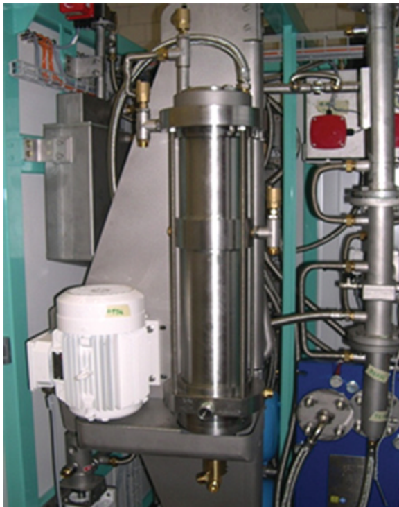
Figure 13.17 Shear Crystallizer in the interior of SeedMaster Compact®. Reproduced with permission of Bühler AG, Switzerland.
